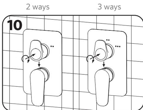
Then assemble the handle and the corresponding wheel.
