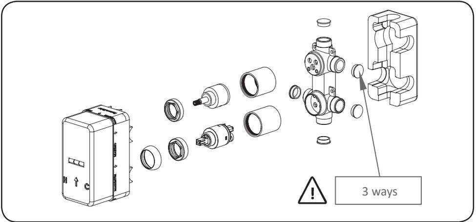
Before installing your new tap, it is essential to clean the installation to eliminate any impurities left in the system that could damage it. We recommend installing filters in the supply pipes. All the parts must be removed from their packaging and inspected before installing, in case any of them have been damaged during transport. If the installation and connection instructions are not followed, the product warranty will be void.
