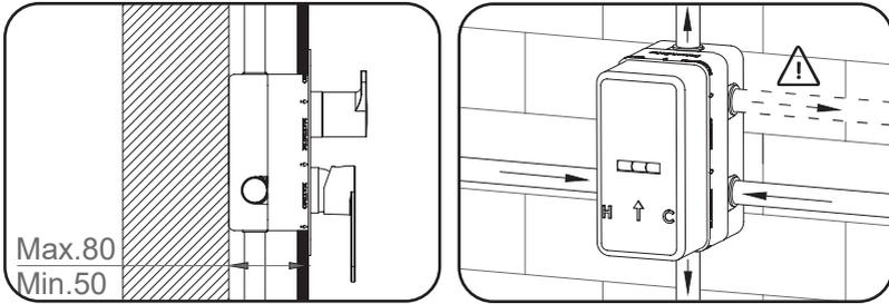
Embedded installation in a brick wall
