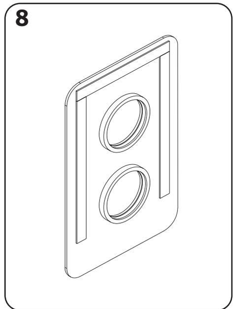
Position the plate chosen according to the model and secure it with adhesive tape.
